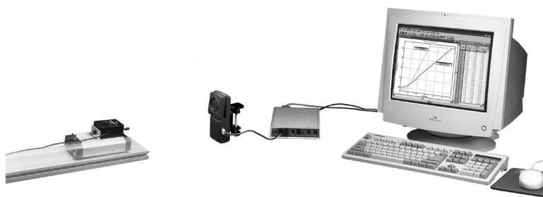
Figure 9.6 Computer-assisted data-acquisition setup showing, from right to left, computer, Vernier ULI and motion detector, PASCO cart on track.
