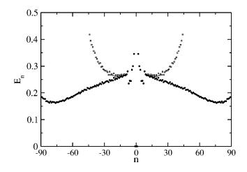
FIG. 5. Fourier modes for N=90 points (open squares) and N=180 points (solid circles) on the perimeter at T=250 K, and  $R=20a_1$ ,  $R_c=40a_1$ .  $E_n$  is measured in atomic spacing units.
