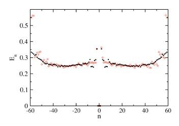
FIG. 4. (Color online) Eigenmodes (open squares) and Fourier modes (solid circles) at T=250 K,  $R=20a_1$ ,  $R_c=40a_1$ .  $E_n$  is measured in atomic spacing units.
