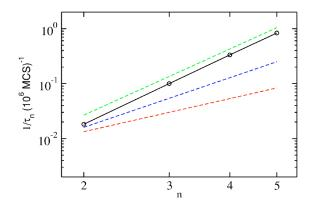
FIG. 8. (Color online) Correlation time  $\tau_n$  vs wave number *n* on a log-log scale. The MC data (black circles) show z=4 which corresponds to step-edge diffusion. The dashed lines represent z=4, 3, and 2 (from top to bottom) dynamic exponents. T=400 K,  $R = 20a_1$ ,  $R_c = 40a_1$ .
