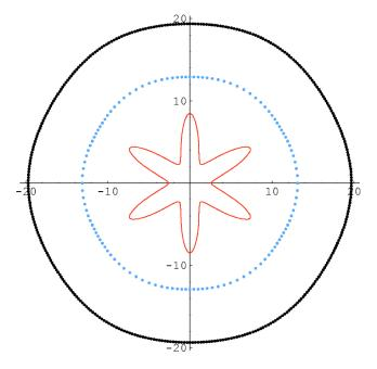
FIG. 6. (Color online) Polar plot of the equilibrium island shape  $R(\theta)$  (outer dots), the relative line tension  $\beta(\psi)$  (inner dots) and the relative line stiffness  $\overline{\beta}(\psi)$  (the innermost curve) in arbitrary units at T=350 K,  $R=20a_1$ ,  $R_c=40a_1$ . (Note the difference between  $\theta$  and  $\psi$ .)
