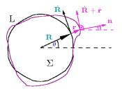
FIG. 3. (Color online) Extension of Fig. 2, showing instantaneous island shape, for analysis of fluctuations. For a particular azimuthal direction,  $\theta$ , the deviation from the equilibrium island shape, r, its derivative with respect to  $\theta$ ,  $\dot{r}$ , the unit vector normal to the instantaneous shape, **n**, and the corresponding angle,  $\psi$ , are all time dependent.
