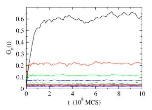
FIG. 7. (Color online) Correlation function  $G_n(t)$  of the Fourier modes for n=2,3,...,10 from top to bottom. T=400 K,  $R=20a_1$ ,  $R_c=40a_1$ .
