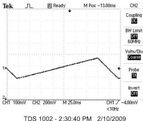
Figure V-3: Setup of the waveform generator ramp signal
