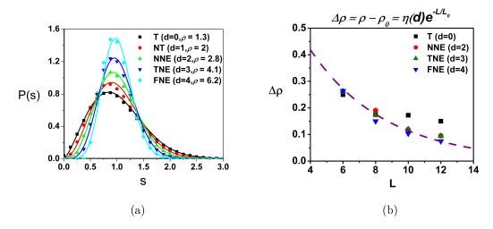
Figure 1: TWDs computed using Monte Carlo simulations: (a) generalized Wigner fits to TWDs of steps with different short-range behavior (b) finite-size effects in interaction strength measurements.
