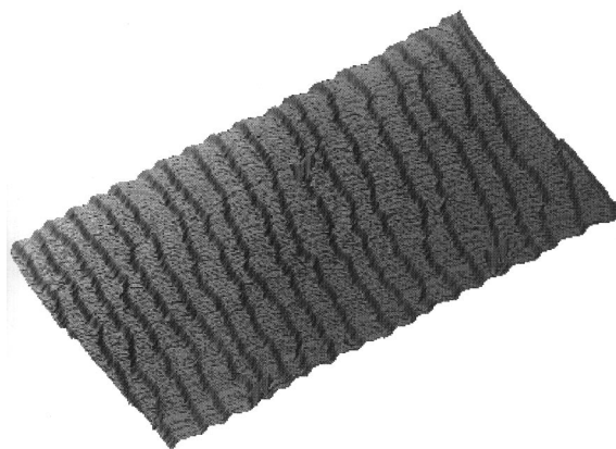
Fig. 2. 2800 \times 2800 \text{ \AA}^2 STM image of a Si(111) surface with a miscut of 1.3^\circ towards the [\bar{2}11] direction after deposition of a third of a monolayer of aluminum at a temperature of 770^\circ\text{C} . After deposition, the sample was quenched to room temperature. The image was taken at room temperature. The surface now consists of an array of single-layer-height steps. The initial positions of the step bunches are no longer visible. The [\bar{2}11] direction is orthogonal to the average step edge direction and in the downhill direction.
